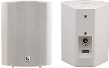
The Galil 5-O On-wall Speaker features a multi-tap power transformer for selecting 8 $\Omega$  (bypassing the transformer) or 70V/100V power settings that are suitable for an array installation. Available in white
